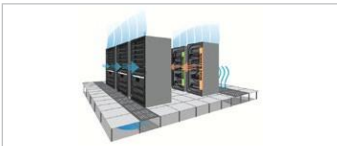
Airflow via in-row cooling units
