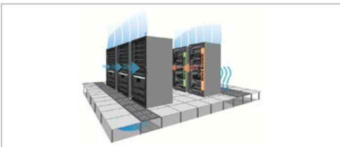
Airflow via in-row cooling units
